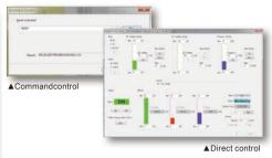
Wavy is an application software that supports sequence creation and the operation for Kikusui power supplies and electronic loads.
